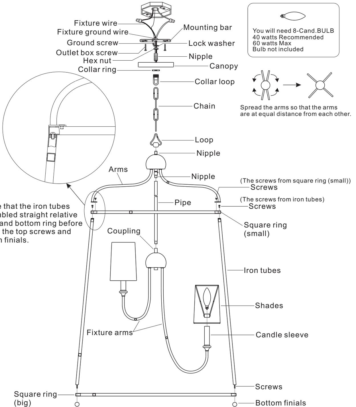
Make sure that the iron tubes are assembled straight relative to the top and bottom ring before tightening the top screws and the bottom finials.
