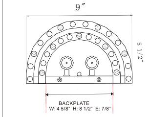
PS:The pattern of the rods to the following outer ring: 2 clear rods + 1 frosted and then repeat, inner ring: 1 frosted +2 clear rod and then repeat.
