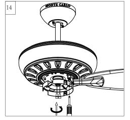
Install the blade assembly to motor using the preinstalled screws. Tighten screws securely. Repeat this process for remaining blade assemblies.
