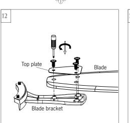
Install blade bracket with blade and top plate as shown above by 3 blade screws provided. Tighten screws securely. Repeat this process for remaining blades.
