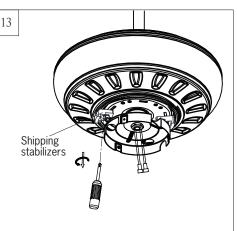
Remove shipping stabilizers from motor assembly.
