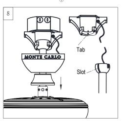
Install ball end of downrod into mounting bracket opening. Align (engage) slot on ball with tab on mounting bracket. **Warning:** Failure to align slot on ball with tab may result in serious injury. **Important**: If using the angle mount, make sure open end of mounting bracket is installed facing the higher point of the ceiling and make sure the ceiling angle is not steeper than 30°. Longer downrod may be necessary allowing the fan blades to rotate without obstructions.
