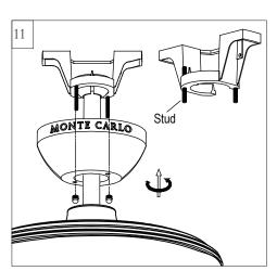
Lift Canopy, allowing the 2 studs to protrude through the canopy. Install knurled nuts provided and tighten the knurled nuts securely. The canopy should adjust for any irregularity in the ceiling or outlet box.
