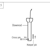
Remove preassembled cross pin and keeper pin from downrod.
