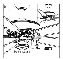
Install witch housing, aligning the holes on switch housing with screw holes on top cover. Reinstall the set screws removed in installation step 15.
