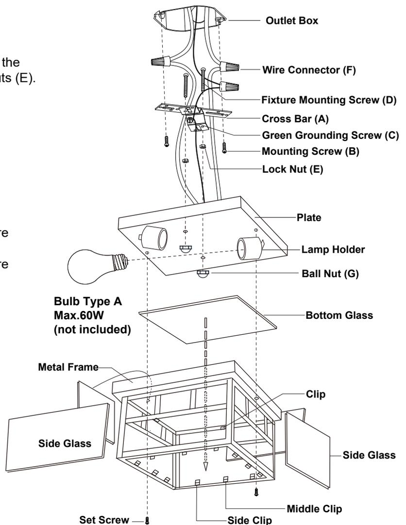
8. Place the side glasses inside the metal frame, then press the clips which on the top of the metal frame and the side clips which on the bottom of the metal frame to secure them.
