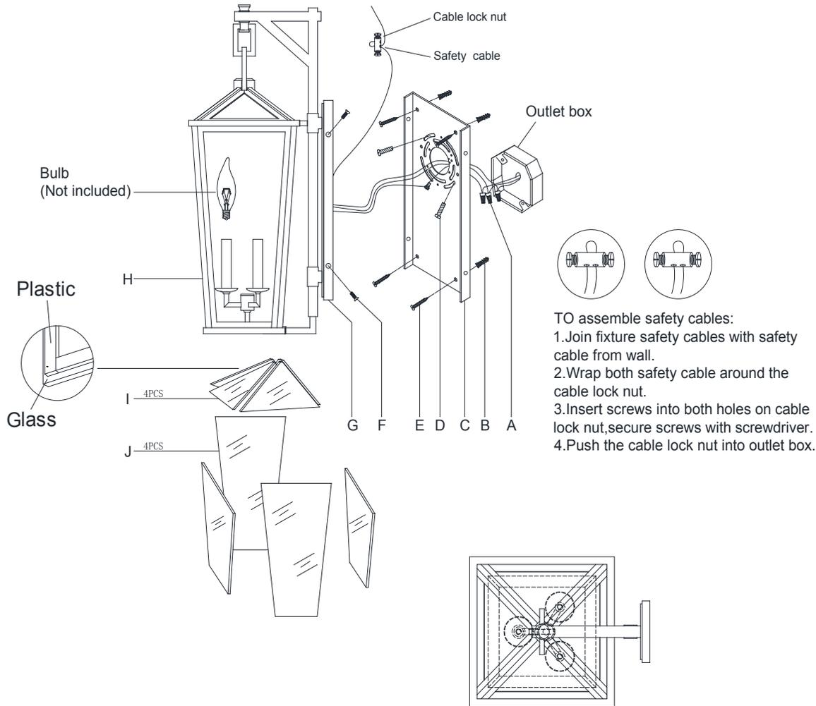
13. Attach backplate (G) to the mounting plate (C) and secure with side screws (F).
