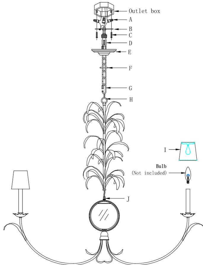
1. Carefully install the fixture leaf column onto fixture thread (J) and secure tightly. Install the crossbar (B) with ceiling loop (D) to outlet box by using mounting screws (C) provided.
