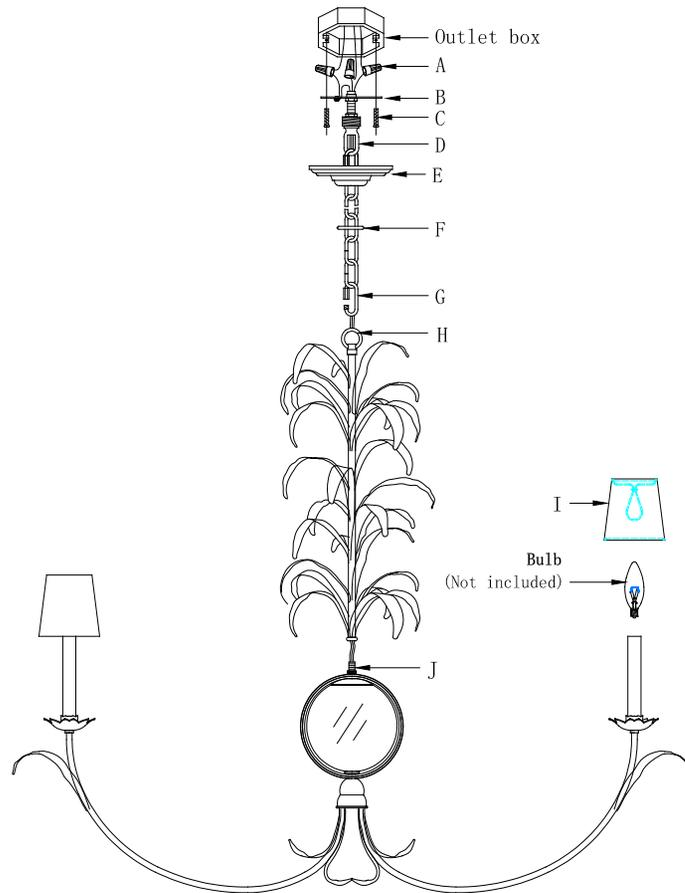
11. Connect the Ground (bare) fixture wire with the ground (usually bare) wire from ceiling box using wire nut (A). If your house does not have ground wire, then attach this wire to the green grounding screw inside of outlet box.
