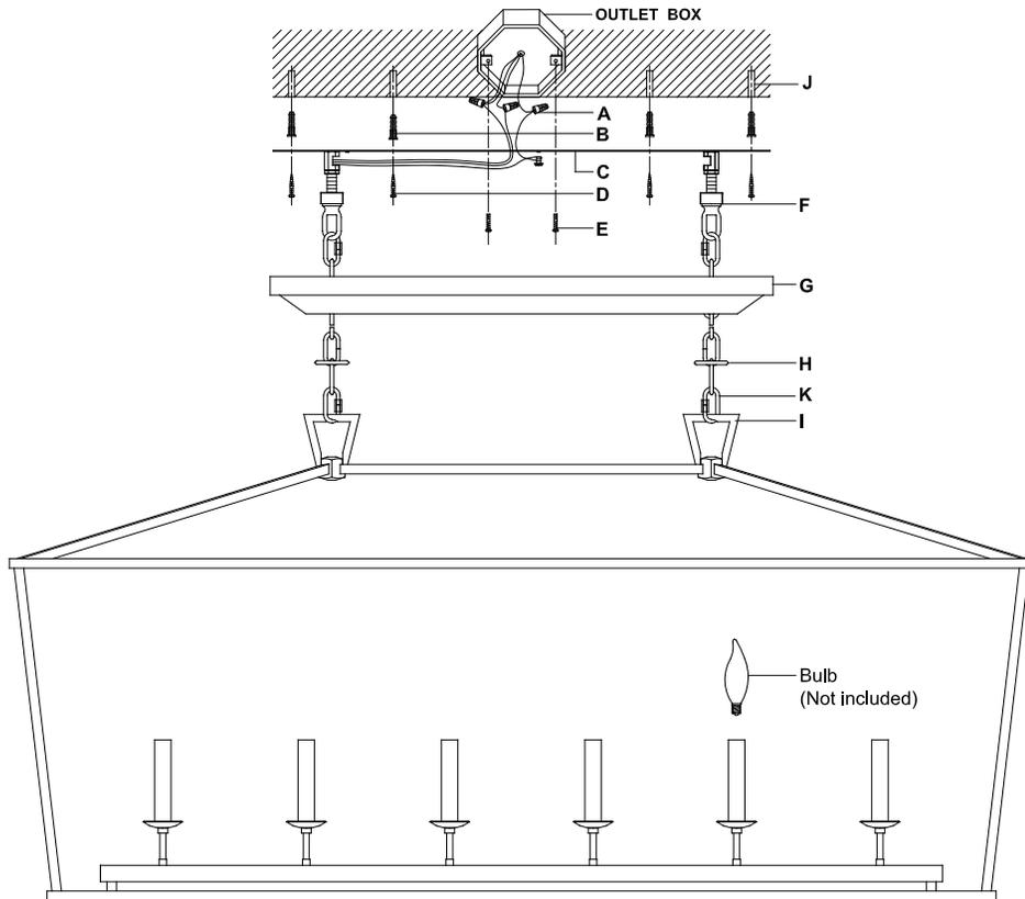
1. Drill 8 holes (J) on the ceiling and make sure the hole distance will match to mounting plate (C) holes
